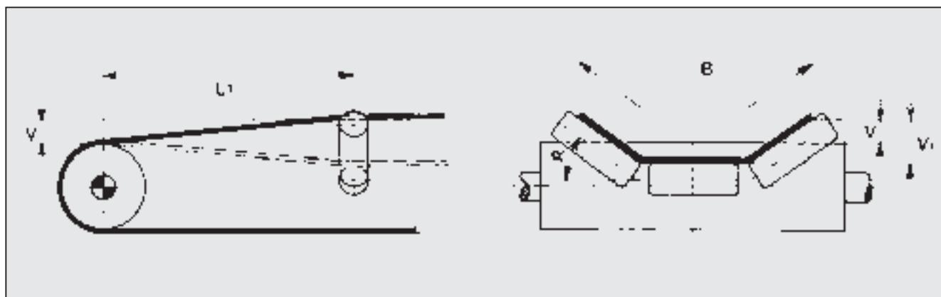
The transition distance is the length of the section between head or tail pulley and the first troughing idler. In some cases, intermediate idlers are placed along the transition distance to favour the passage of the belt from the flat to the trough shape.
